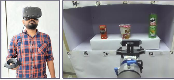
Fig. 1: (left) Operator wearing the Head Mounted Display along with handheld controllers. (right) A mock retail shelf unit along with the robot end-effector. It contains 3 distinct grocery items and the operator is tasked with picking them via teleoperation.
