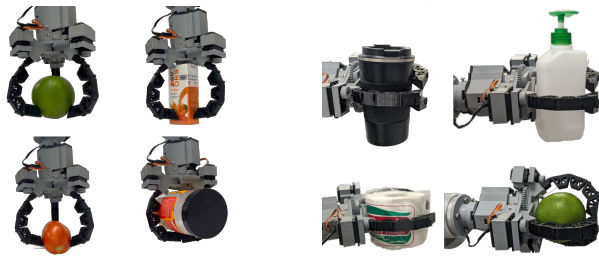
(a) Top-Down grasp of retail objects with spherical (left-top, right-top, left-bottom) and cylindrical(right-bottom) configuration (b) Sideways grasp of retail items in cylindrical (left-top, right-top, left-bottom) and spherical (right-bottom) configuration
