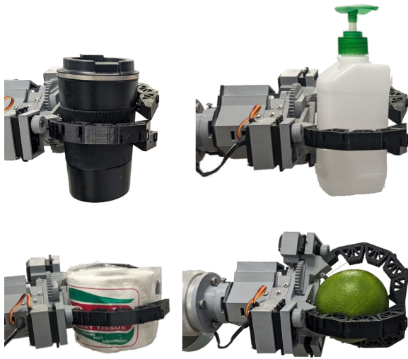
Fig. 9. Sideways grasp of retail objects using soft gripper in cylindrical configuration (left-top, right-top, left-bottom) and spherical configuration (right-bottom)
