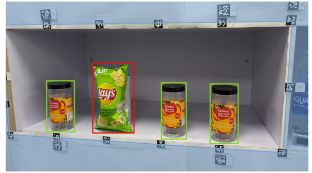
Fig. 7. Shelf detection module masking out the part of the image outside the rack (blue tint). Anomaly detection module localizing the anomaly within a rack (red bounding box)
